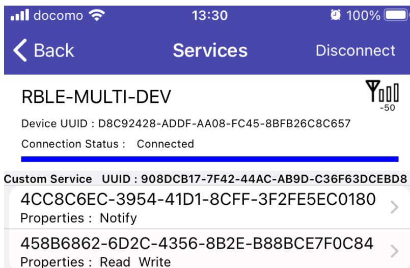
Figure 12-10 Detected GATT service and characteristics
